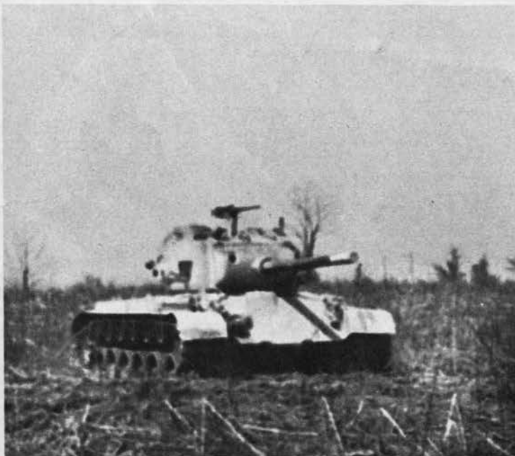
Heaviest U. S. tank will be the 42-ton M-26. With heavy armor and a big 90-mm. gun, it should be in approximately same fighting class as Nazi Tiger. Its massive turret sits forward on the low hull.
